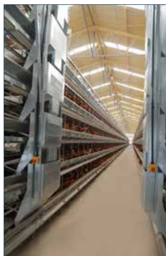
Figure 9. Hopper feeders drop feed directly into the feed trough. Image courtesy Alaso.
