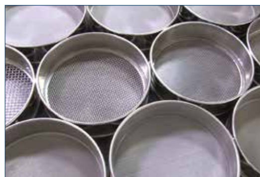
Figure 3. Sieves of varying sizes used to separate a mash feed sample by particle size. Image courtesy Gilson Company, Inc.
