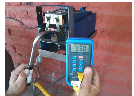
Pyrometer indicating proper blade temperature of 650°C.
