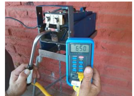
Pyrometer indicating proper blade temperature of 650°C.
