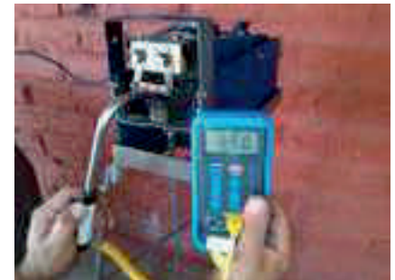
Pyrometer indicating proper blade temperature of 650°C.
