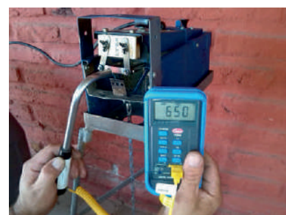
Pyrometer indicating proper blade temperature of 650°C.
